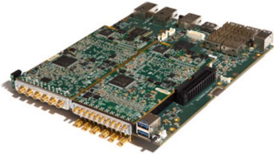
Figure 1. SBC-Duo Motherboard (XMC modules sold separately)
