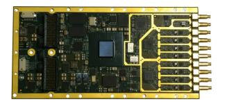
The XA-RX is an XMC IO module featuring eight 16bit, 125 MSPS A/D channels designed for high speed imaging, ultrasound and MRI, quadrature radio receivers, diversity radio receivers, and test equipment.
