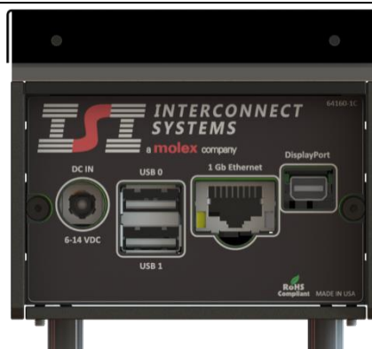
Figure 3. Rear view of SBC-Nano system in a chassis.
