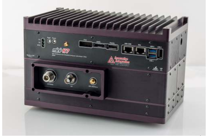
Figure 2. Mini-K7 with optional signal conditioning and touch screen trays, front right
