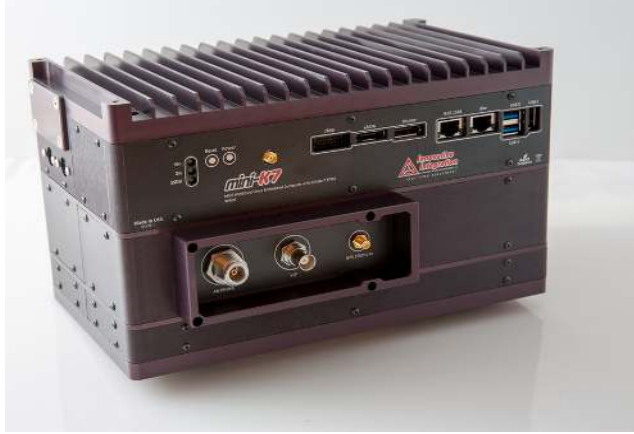
Figure 1. Mini-K7 with optional signal conditioning and touch screen trays, front left
