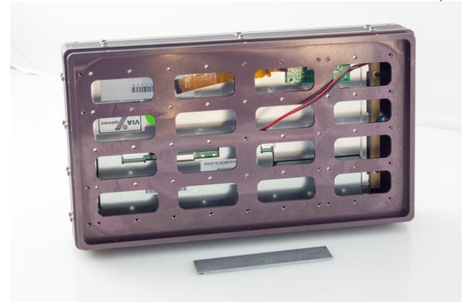
Figure 8. Optional touch screen tray (bottom), P/N 30402
