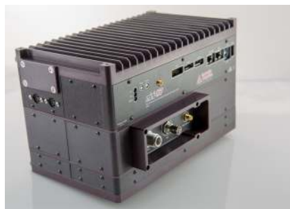
Illustration 1: SW-K7 atop optional RF receiver and touch screen trays.
