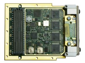
The FMC-SDF module features four simultaneously sampling ADCs and a dual output DAC. High resolution sigma-delta ADCs and high-resolution DACs support high dynamic range applications such as audio, ATE, and seismic data acquisition.
